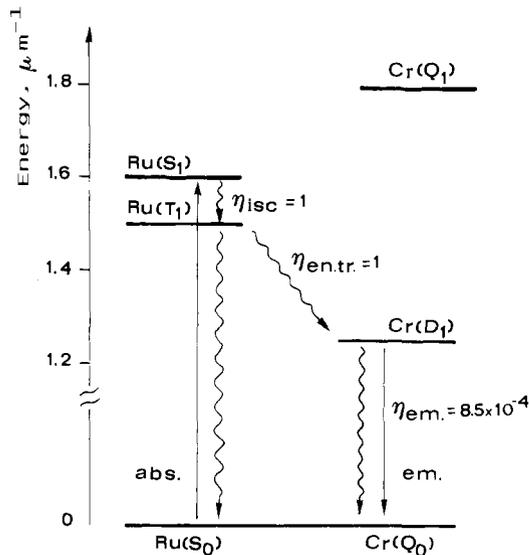
Figure 5. Energy level diagram and photophysical processes of  $[\text{NC-Ru}(\text{bpy})_2\text{-NC-Cr}(\text{CN})_5]^{2-}$  (see text).
