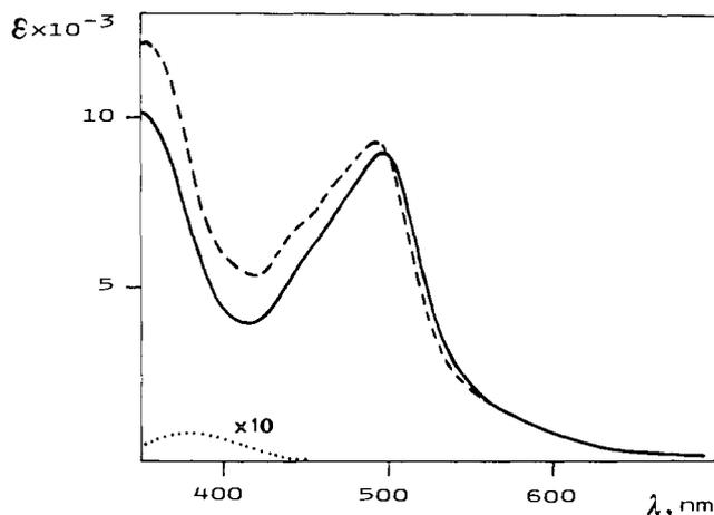
**Figure 1.** Absorption spectra of [NC-Ru(bpy)<sub>2</sub>-NC-Cr(CN)<sub>5</sub>]<sup>2-</sup> (continuous line), [(CN)<sub>5</sub>Cr-CN-Ru(bpy)<sub>2</sub>-NC-Cr(CN)<sub>5</sub>]<sup>4-</sup> (broken line), and Cr(CN)<sub>6</sub><sup>3-</sup> (dotted line, ×10 expansion) in DMF.
