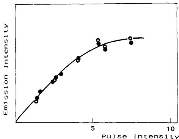
Figure 4. Dependence of the initial ( $t = 50$  ns) emission intensity on the intensity of the exciting laser pulse.  $[\text{NC-Ru}(\text{bpy})_2\text{-NC-Cr}(\text{CN})_5]^{2-}$  (●);  $[(\text{CN})_5\text{Cr-CN-Ru}(\text{bpy})_2\text{-NC-Cr}(\text{CN})_5]^{4+}$  (○). Units of pulse intensity correspond to concentrations of absorbed photons in  $\text{einstein-L}^{-1} \times 10^{-5}$ . Complex concentration:  $2 \times 10^{-5}$  M.
